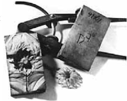
Normally a mold release agent is not needed, although some workers prefer to use talcum powder or a silicone or Teflon® spray. If talcum powder is used, avoid a buildup of powder in the mold cavity, cleaning it if necessary with an air gun or a soap and water solution.
