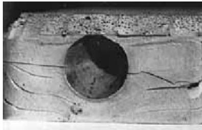
**This mold shows obvious signs of not having been packed fully enough. Separate layers of rubber are easily visible, as are air bubbles.**
